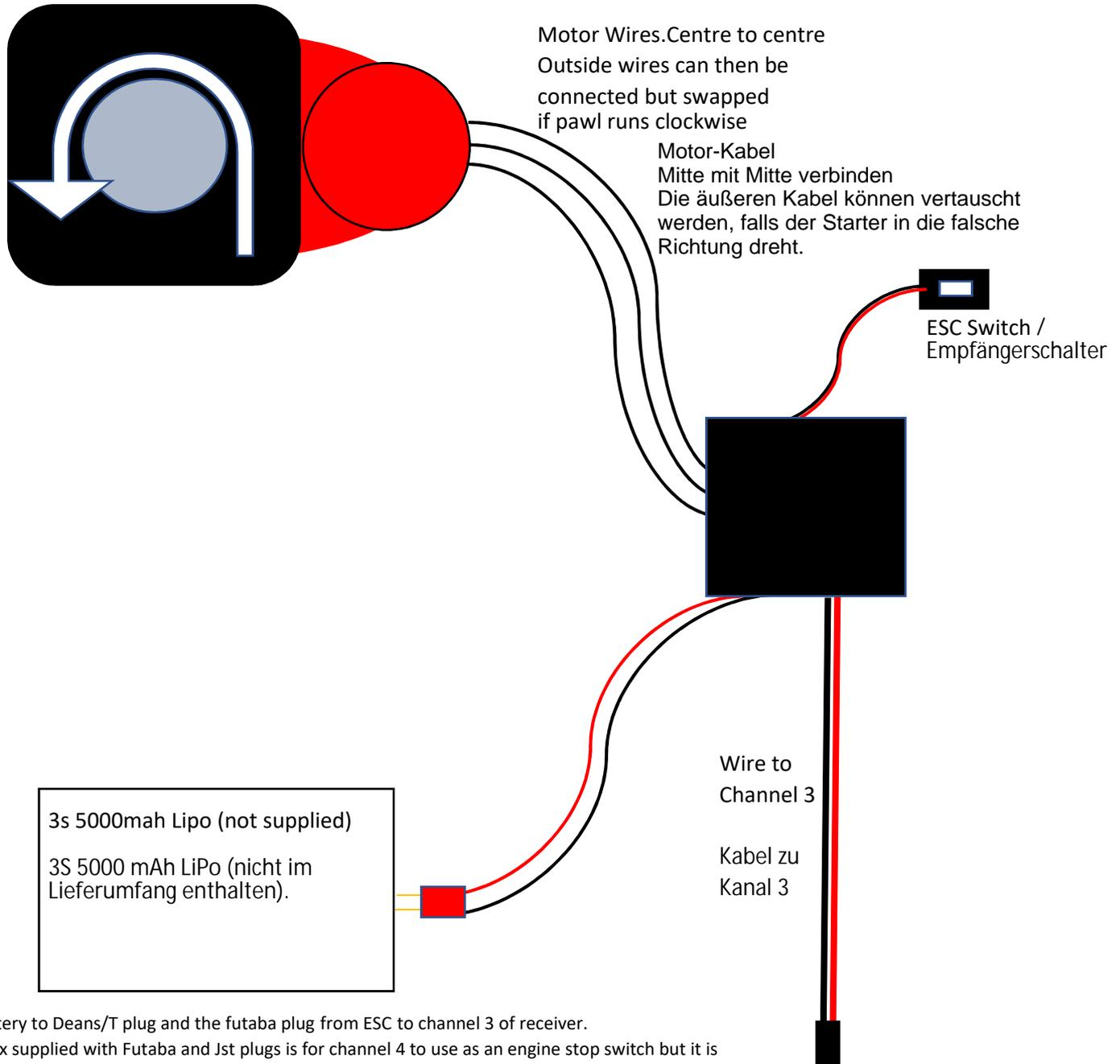
Connect battery to Deans/T plug and the futaba plug from ESC to channel 3 of receiver.
